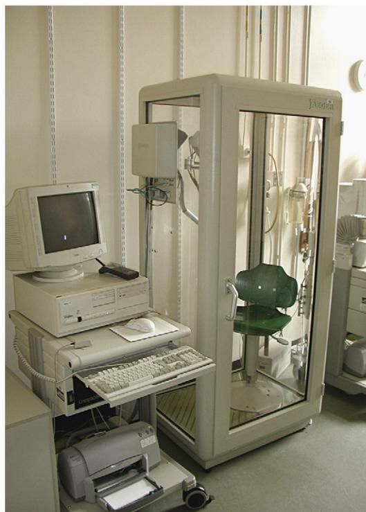
Figure 1 Body box plethysmograph used for pre-flight testing.
